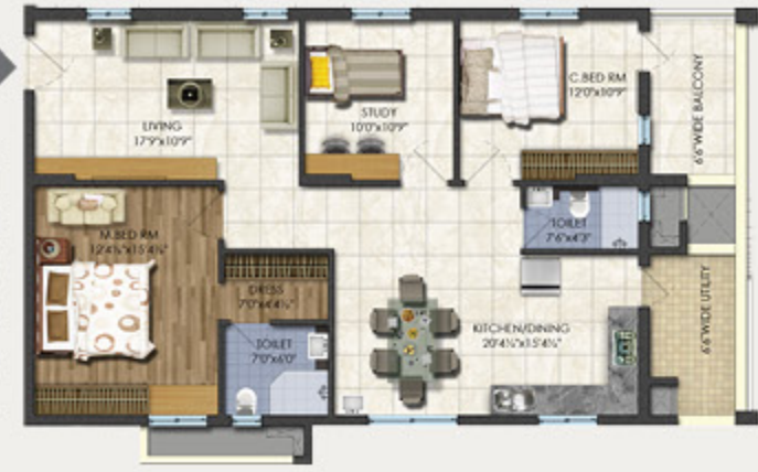
TYPICAL FLOOR PLAN Type -N Flat No.20 (West Facing) 2BHK + Study 1665 sft.
