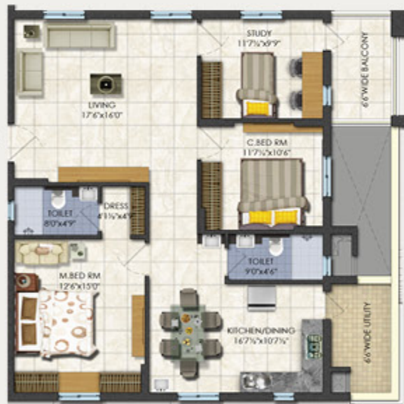
TYPICAL FLOOR PLAN Type -O Flat No.22 (West Facing) 2BHK + Study 1665 sft.
